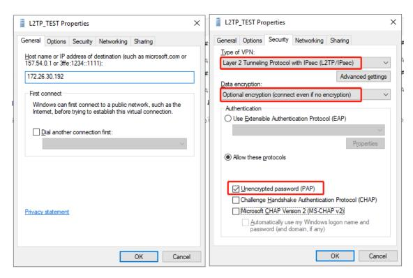
e If IPsec encryption is enabled on the server, select **CHAP** and **MS-CHAP v2** as the identity authentication protocols and click **Advanced settings**. In the dialog box that appears, configure the pre-shared key the same as that on the server. After completing the configuration, click **OK**.
