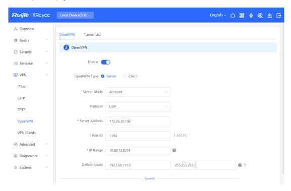
b Turn on Enable to enable the OpenVPN function, set OpenVPN Type to Server, select a server mode and protocol, enter the port number (1194 by default) and server address (external IP address of the local device), and click Save.
