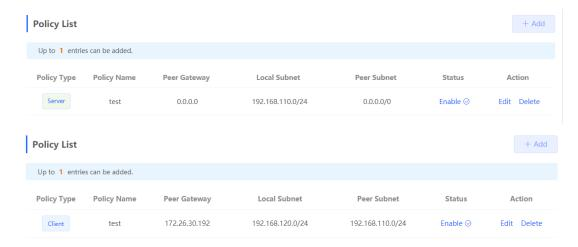
(3) Check whether the WAN IP address of your HQ EG is a public IP address. If not, you need to configure DMZ or port mapping (UDP 500 and 4500 used as IPsec VPN port) on your egress gateway and set **Local ID Type** to **NAME** on HQ and branch gateways.
