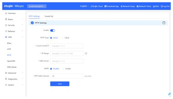
b Turn on the PPTP function, set PPTP Type to Server, enter the local tunnel address, address pool IP address range, and DNS server address, specify whether to enable MPPE encryption, and click Save.
