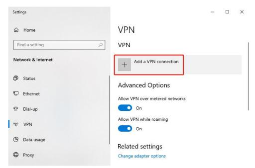
Click Add a VPN connection. In the dialog box that appears, set VPN provider to Windows and VPN type to Point to Point Tunneling Protocol (PPTP), enter the connection name and server address or domain name, and click Save.
