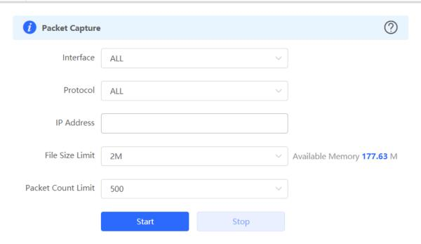
Packet capture can be stopped at any time. After that, a download link is generated. Click this link to save the packet capture result in the PCAP format locally. Use analysis software such as Wireshark to view and analyze the result.
